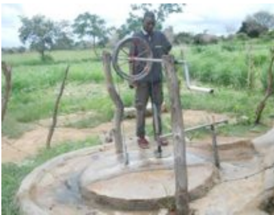
Figure 7: Functioning rope pump Figure 8: Rope pump in the process of repair (replacement of rope, requires replacement of rope, cleaning of the well and replacement of well cover) Sioko village, Choma. Chinyengele village, Magoye.
